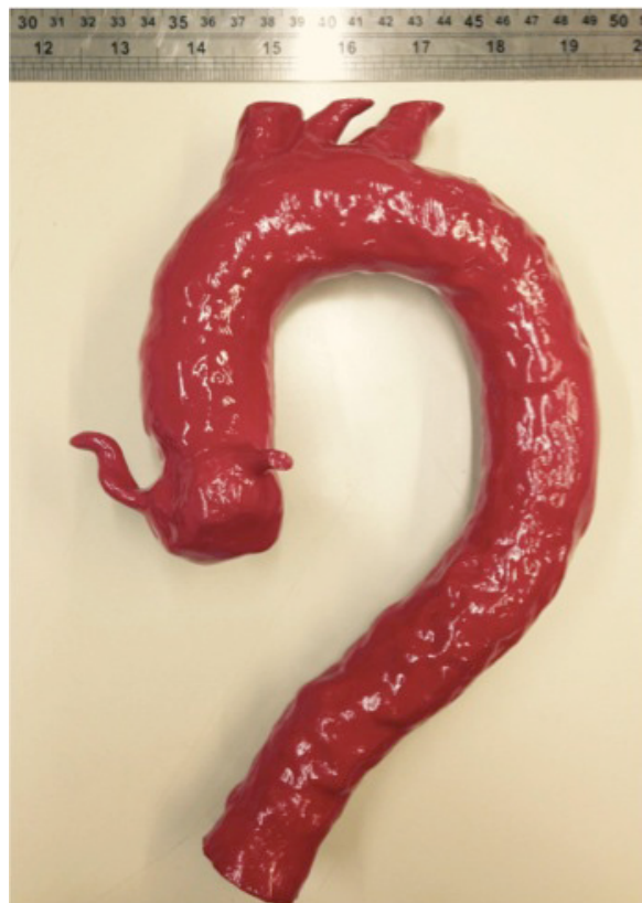
Figure 1 – Three-dimensional aortic model. Model in ABS-M30 Affordable FDM thermoplastic material (Stratasys, USA).
