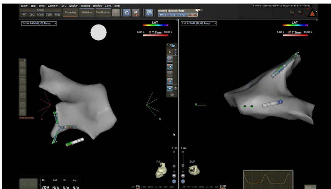
**Video 3** – High definition anatomic reconstruction of LA and PVs. With the multipolar mapping catheter, the anatomic acquisition is obtained by sequentially moving the mapping catheter, while the ablation catheter is parked in the mitral annulus. Two different views are shown (posterior and superior). Access the video here: <https://bit.ly/2XWhIbE>.
